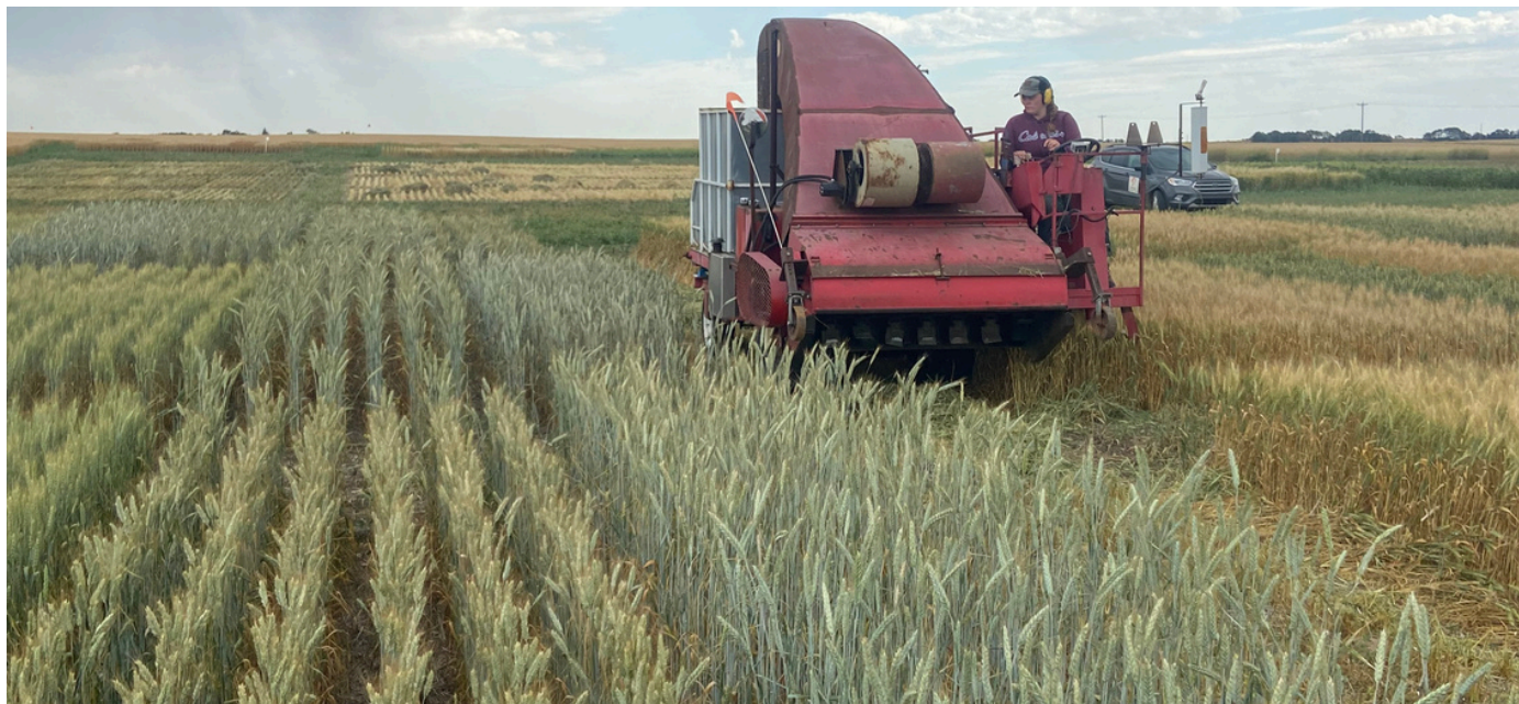
Figure 9. Updated forage harvester with new fans to reduce plugging. This harvester is used for most of our whole plot silage harvesting.
