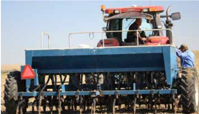
Precision seeding will ensure the seeds are placed at the correct depth, and allow for most effective soil to seed contact.
